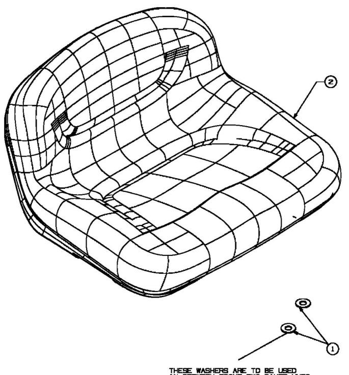
THESE WASHERS ARE TO BE USED IN BETWEEN FRONT TWO RIVET NUTS IN BOTTOM OF SEAT PAN AND SEAT MOUNTING PLATE.
